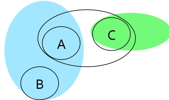
A and B have closer centroids than A and C, but closest points are from A and C.
